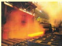
beginning of hot-rolling operations at 1200°C
