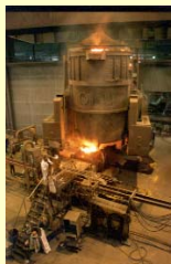
a 200T ladle during casting operations
